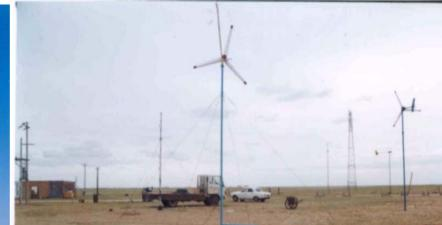
Field-Test of Wind Turbines All wind-turbines must pass a one year field reliability test.
