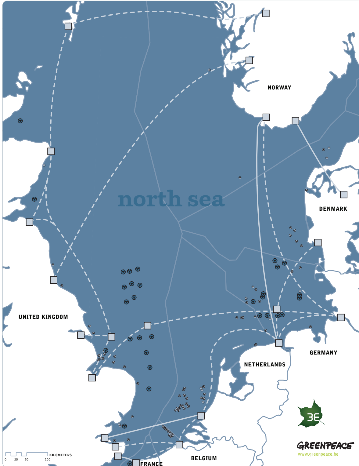
figure 4.3: offshore grid topology proposal and offshore wind power installed capacity scenario
