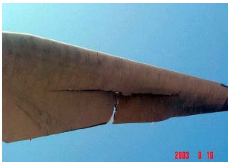
Crack on a blade of wind generator
