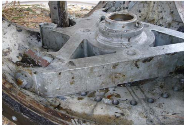
Damaged V-poking fork and connecting rod
